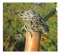
the SAP and the Control person were notified and the defective earth was replaced and recovered safely allowing work to continue.
