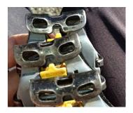
Closer inspection suggested the cracks may be splits in the fold of metal which may have formed due to wear. Over time as the buckle has worn it has developed a small lip/burr on the edge. It appears this is actually a small split or gap in this surface burr as opposed to a crack in the buckle.
