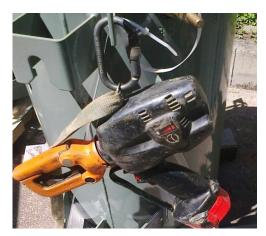
An investigation is currently in progress to determine all of the facts and the root cause, but one area identified is that the battery being used in the crimping tool had defective locking clips that are designed to secure the battery into the tool.
