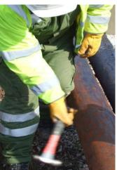
Along with the well documented generic recommendations below it would be good practice, where a new pole is to be installed, to carry out a thorough visual inspection and a hammer test prior to a new pole being dressed and erected.
