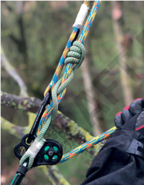
9.2.1a Using a slack-tending pulley beneath the friction hitch.
