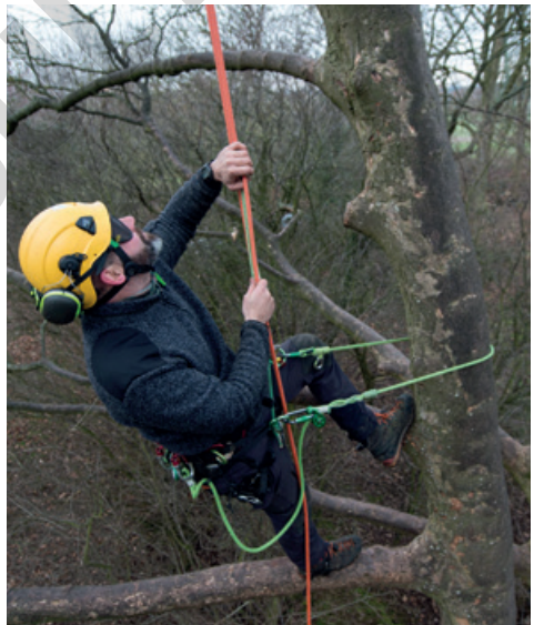
9.5.3c Lanyard used to provide backup.
