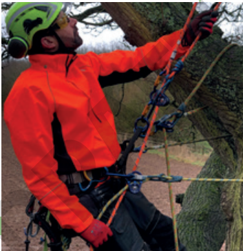
8.1.1e Primary and backup systems in place with the addition of a lanyard to allow two permanent connections to be maintained.
