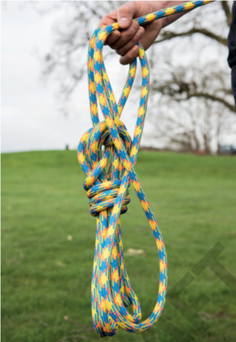
7.3.2 A coil allowing the rope to unravel once thrown.
