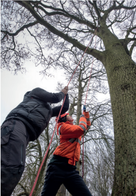
11.3.2 Proof loading anchors from ground level.
