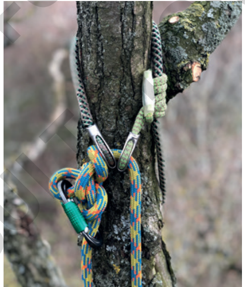
11.7.3 An alpine butterfly incorporating an autolocking component used as a knot blocker.
