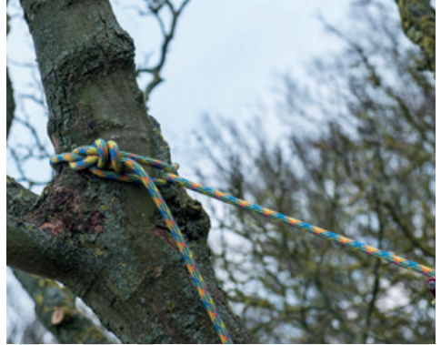
11.7.1 A running bowline used to form a canopy anchor.
