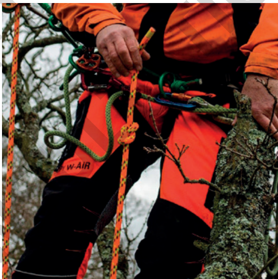
10.2a A rope length check performed by the climber using the other end of the primary system, with a stopper knot.
