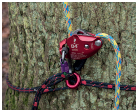
11.6.1 Basal anchor incorporating an industrial belay device.
