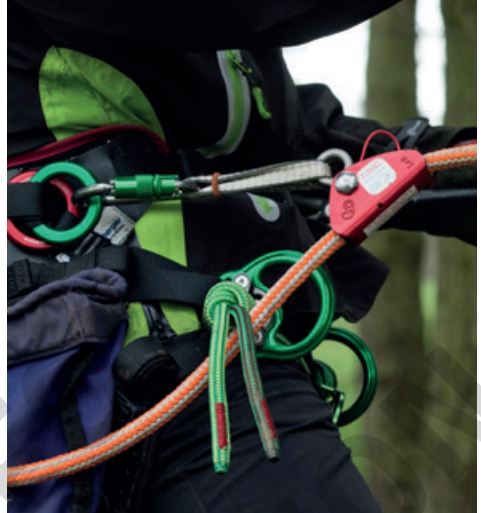
14.2.4 Cut away or soft link included as part of the lanyard system.
