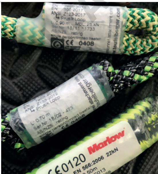
14.1.3 Friction cord selected against criteria a–d.
