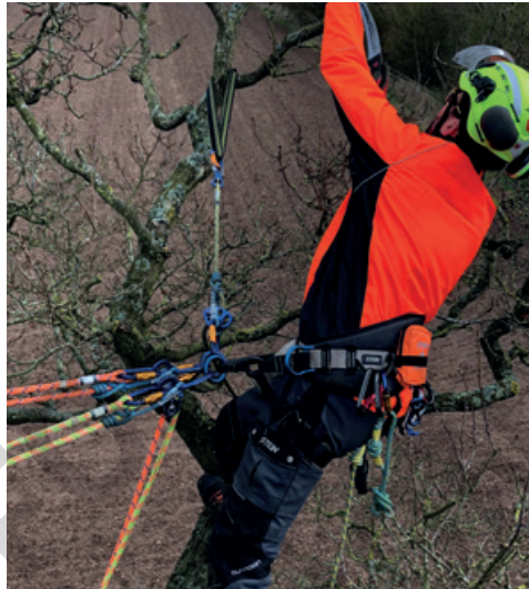
11.9.3c A tape sling used to extend the length of the climber's lanyard.
