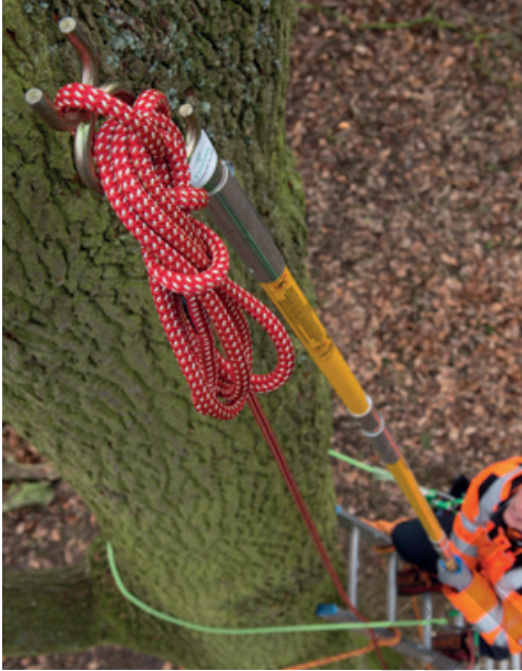
7.5.1 Using an extendable pole to assist with rope installation.
