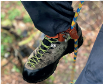
8.1.1f Incorporating a foot ascender helps facilitate an ascent.
