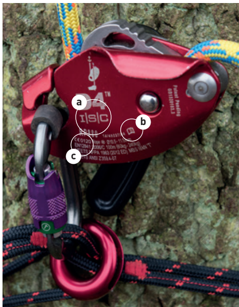
13.5.3 Basal anchor incorporating an industrial belay device. a = manufacturer. b = symbol for instruction manual. c = EN12841 reference
