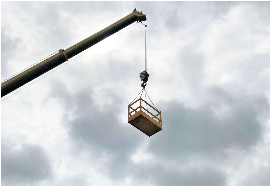
A personnel carrier suspended from a crane.
