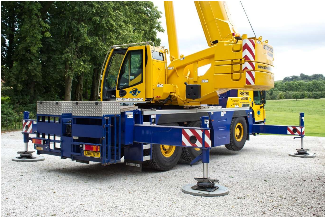
Example of a fully rigged crane
