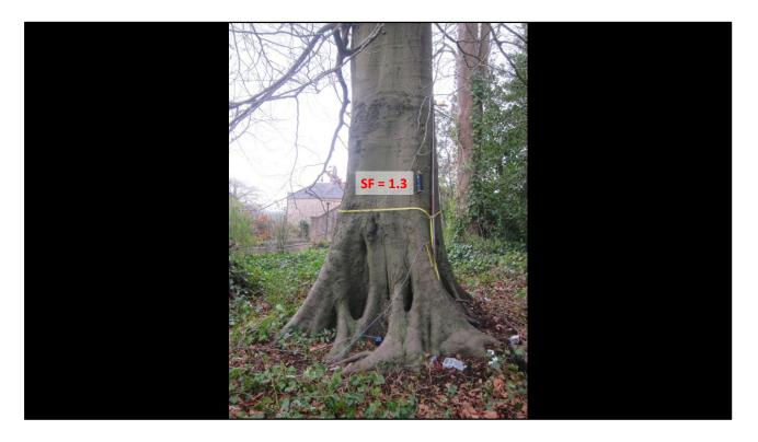
This tree fails the test with significantly reduced safety factors, that fall below the minimum threshold of 1.5, at around 1.0-1.2 m on the stem.
