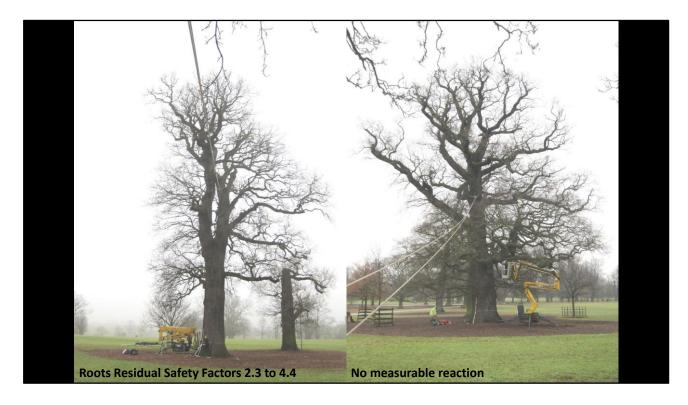
The majority of residual safety factors for uprooting for the tree on the left were between 3.0 and 3.5 with the lowest safety factor for uprooting of 2.3.
