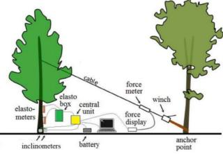
The setup for Pulling Test for both root and trunk evaluation.
