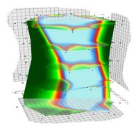
The Arborsonic 3D is a Sonic Tomography System, using up to 32 sensors enabling detailed assessment of trees suspected of decay or defect.
