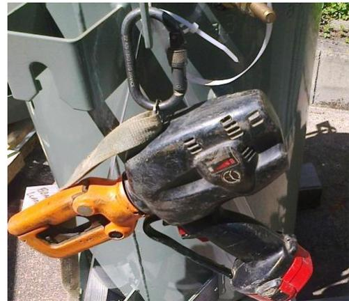
An investigation is currently in progress to determine all of the facts and the root cause, but one area identified is that the battery being used in the crimping tool had defective locking clips that are designed to secure the battery into the tool.
